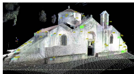
Interior (left) and exterior (middle) images of Panagia Kera, and 3D point cloud of exterior surfaces of the monument (right) acquired with laser scanning.
